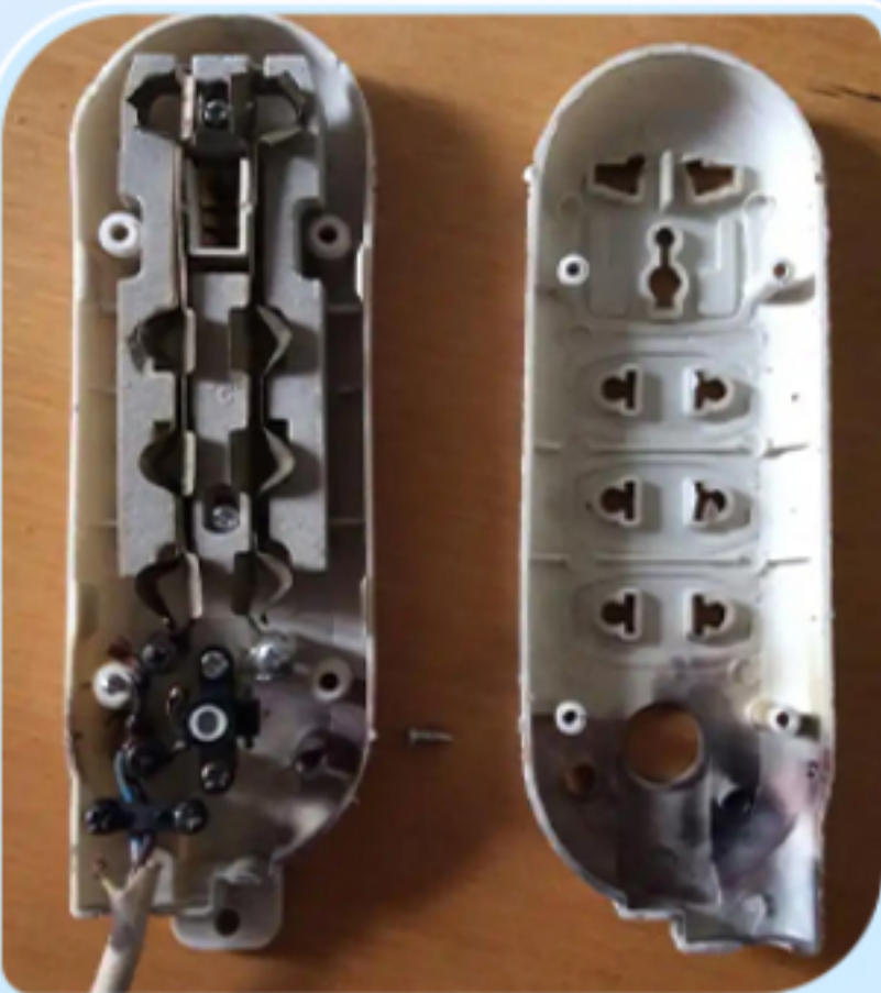
Poor Contact between Plugs and Sockets, Overheating at Contact Areas Leading to Fires
