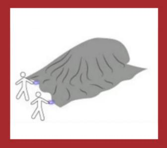
6. REMOVE THE FIRE BLANKET FROM THE CAR AND MOVE AWAY FROM THE VEHICLE.
