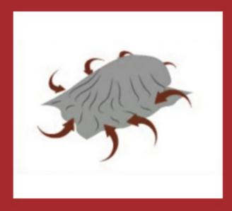
4. ENSURE THE FIRE BLANKET COVERS THE FIRE COMPLETELY AND TIGHTLY TO PREVENT OXYGEN FROM ENTERING, ACHIEVING OXYGEN ISOLATION FOR EXTINGUISHING THE FIRE.
